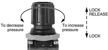
**Caution:** The vacuum regulator constantly sucks in a minute amount of atmospheric pressure air to maintain a balance. As a result, be careful to avoid blocking the body's inlet for outside air. Pressure cannot be set when the inlet hole is blocked.
